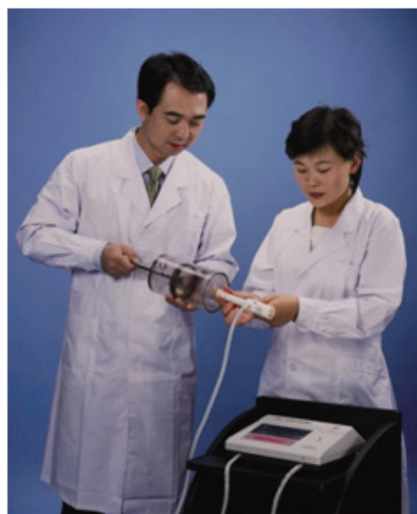
Figure 1-2 Calibration of electronic spirometer
